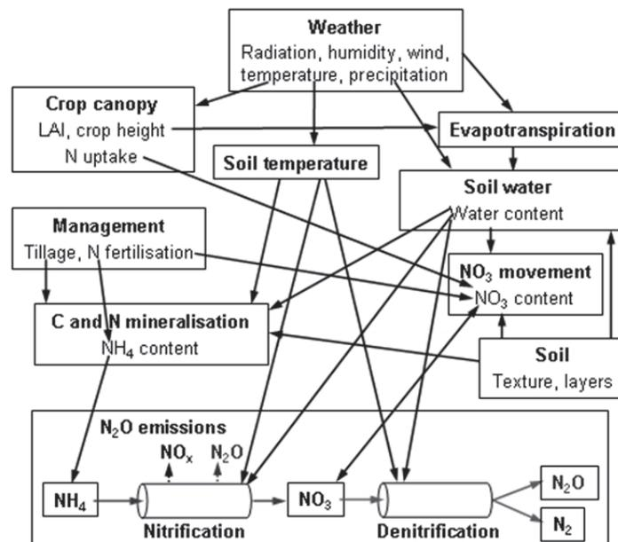
Figure 1: Simplified scheme of the coupled dynamic soil-plant-atmosphere model with processes and variables influencing N<sub>2</sub>O emissions by nitrification and denitrification
