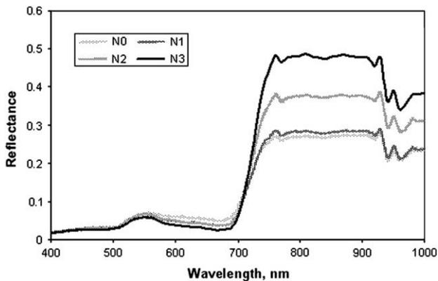
**Fig. 4 – Canopy reflectance spectra of four differently fertilized OSR plots of one block on 29 April 2005: 0 kg N ha<sup>-1</sup> (N0), 80 kg N ha<sup>-1</sup> (N1), 160 kg N ha<sup>-1</sup> (N2) and 240 kg N ha<sup>-1</sup> (N3).**
